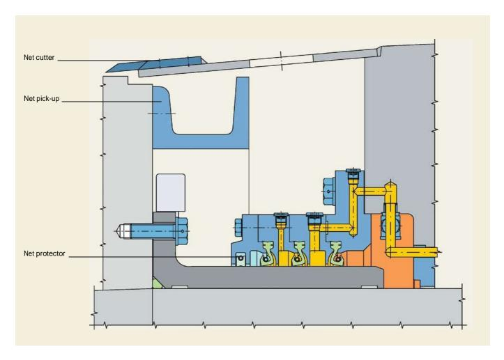
There are three options for protecting the aft seal from damage caused by fishing nets or lines. All three options can be used individually or in combination:
